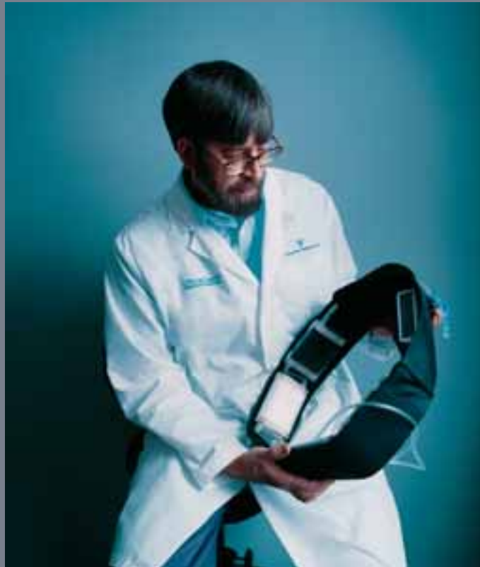
Smaller and better: Harold F. Sandford, PhD, a member of Norma Ofsthun's research team, with a prototype of the wearable artificial kidney. The final product should work more efficiently than previous technologies and remove numerous toxins from the blood, much like a real kidney.
